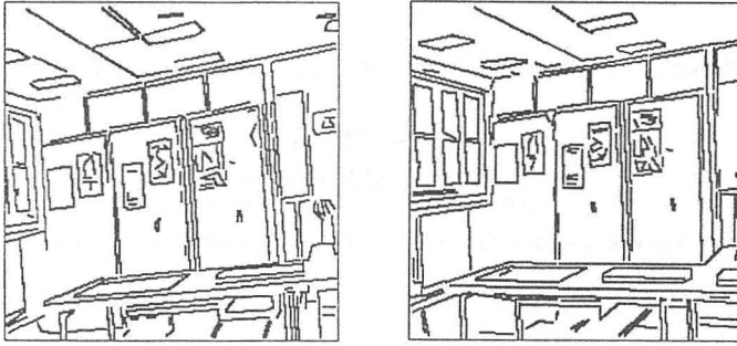
Figure 1: Example of segment images extracted from two views of the same scene. The left image has 323 segments and the right one has 314 segments.
