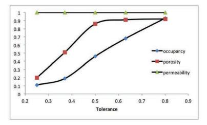
**Figure 2**. Occupancy, porosity, and permeability versus tolerance. Frontier on a grid network ( $\delta = 90\%$ ).
