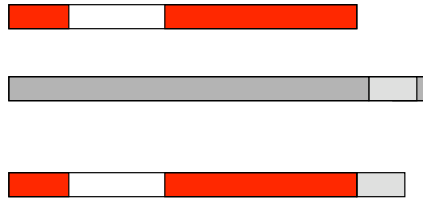
Figure 3. XOA crossover. If there is no length overlap between code selected in the second parent and the first parent (top), the selected code fragment is appended to the whole of the code from the first parent. (That is, the middle portion of the first parent is not removed.)
