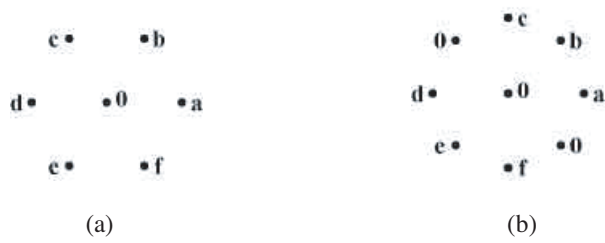
Figure 15. (a) Hexagonal star graph (seven vertices) and (b) nine-vertex star graph (0s showing the empty center and two unnecessary positions).
