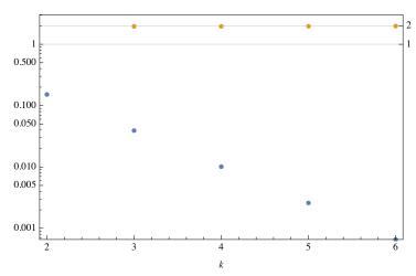
• max-norm of continuous-discrete normal equation solution,  $m = 2^k$  • calculated convergence order
