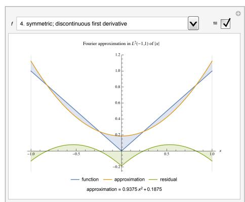
This shows the Fourier approximation of a sample set of functions.
