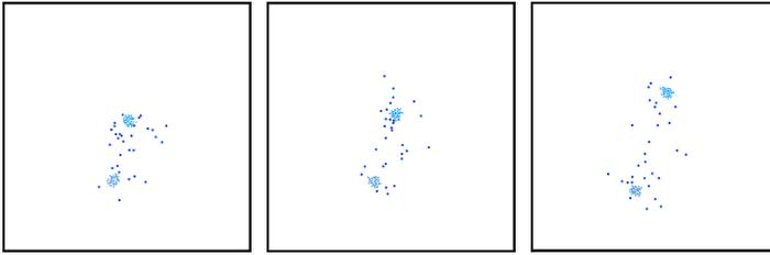
**Figure 8.** The use of the motion algorithm given in equations (41) and (42) to move two clusters apart to a predetermined relative distance. 100 pucks and 50 robots are used with the robots and pucks having radii of 1 and 0.5 units respectively. Information on the specific  $f$ ,  $h$ , and  $g$  functions used can be found in [7].
