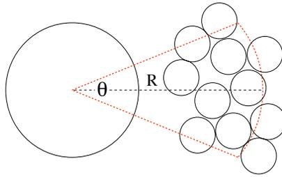
**Figure 3.** A robot approaching a cluster of building material. For simplicity, we assume that the cluster is circular. The robot will then estimate the cluster size by measuring what it perceives as the diameter of the cluster.
