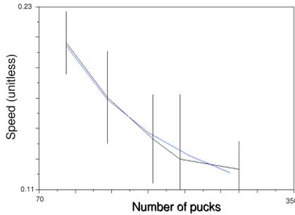
**Figure 6.** The cluster speed as a function of its size, holding the density of robots  $\alpha$  constant. The predicted behavior of the cluster speed matches well with the observed behavior.
