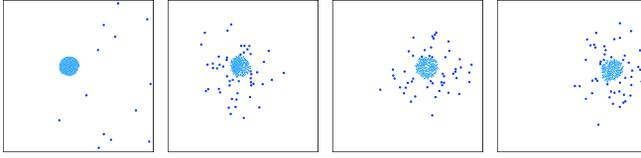
**Figure 5.** The movement of a cluster. 200 pucks and 50 robots are used with the robots and pucks having radii of 1 and 0.5 units respectively. Information on the specific  $f$ ,  $h$ , and  $g$  functions used can be found in [7].
