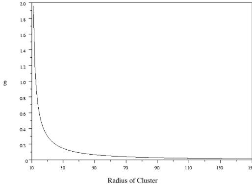
**Figure 1.** A form of the  $g$  functional that is suitable<sup>2</sup> for constructing a single cluster. Robots employing a behavior which creates this  $g$  form will build a single cluster from any initial distribution.
