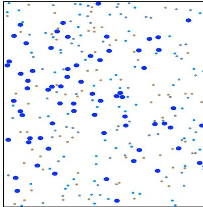
**Figure 2.** A screenshot of the simulation. The larger circles represent robots while the smaller circles represent pucks. 200 pucks and 50 robots are used with the robots and pucks having radii of 1 and 0.5 units respectively.
