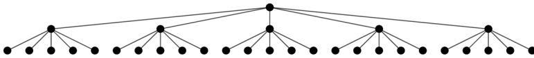
Figure 5. Hierarchy network ( k -ary tree) with 30 vertices and an SOC of five, and thus almost three full levels.
